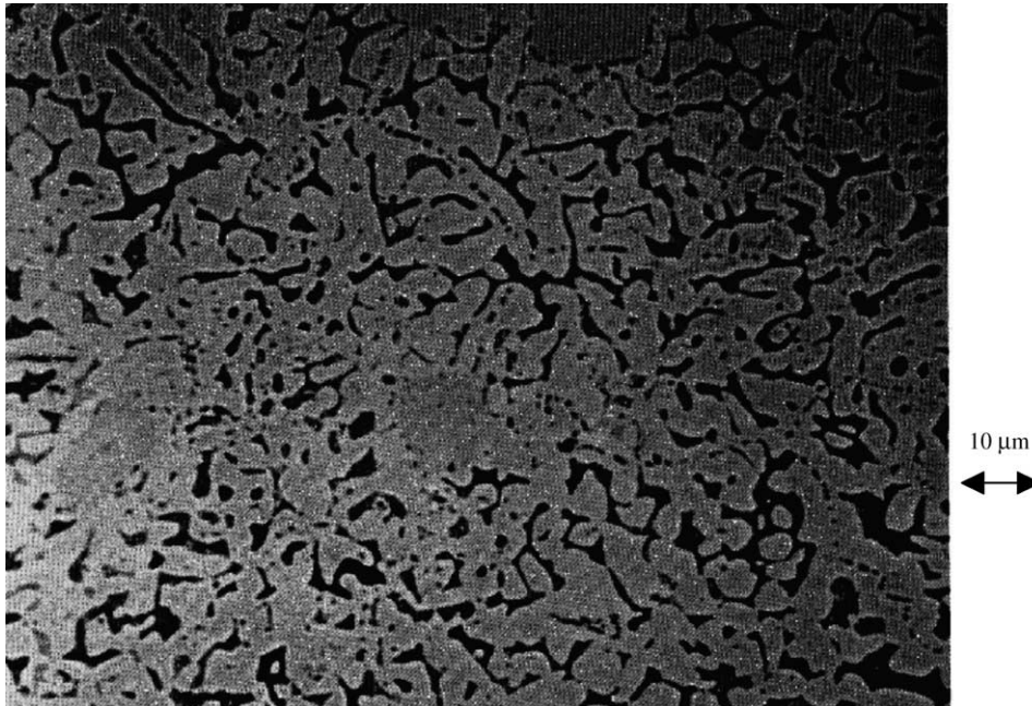
Fig. 1. Microstructure of unirradiated U_{0.31}ZrH_{1.6} (from [3]). Black areas are uranium metal; ZrH_{1.6} is gray.
